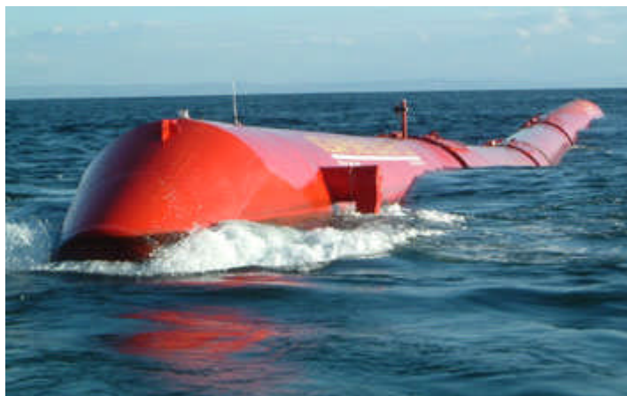
The Pelamis system, set for deployment next year, generates electricity when waves bend its pontoons, pushing hydraulic fluid through a motor.
